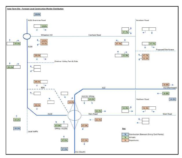
Figure 6: Construction Worker Trip Distribution (Solar Farm Site, Local Staff)
