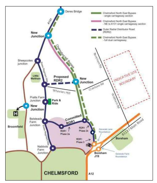
Figure 9: Highway Improvement Works in the vicinity of the Boreham Interchange Source: Chelmsford Local Plan SOCG 22 (November 2018)
